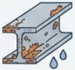
3. Structural Deterioration / Corrosion
